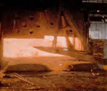
THE FORKLIKE PEEL deftly enters blazing furnace to lift out a red-hot steel blank.
